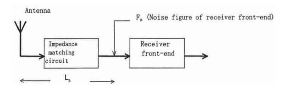
From Fig. 1, field strength equivalent to the receiver intrinsic noise (Eri) is expressed by:
