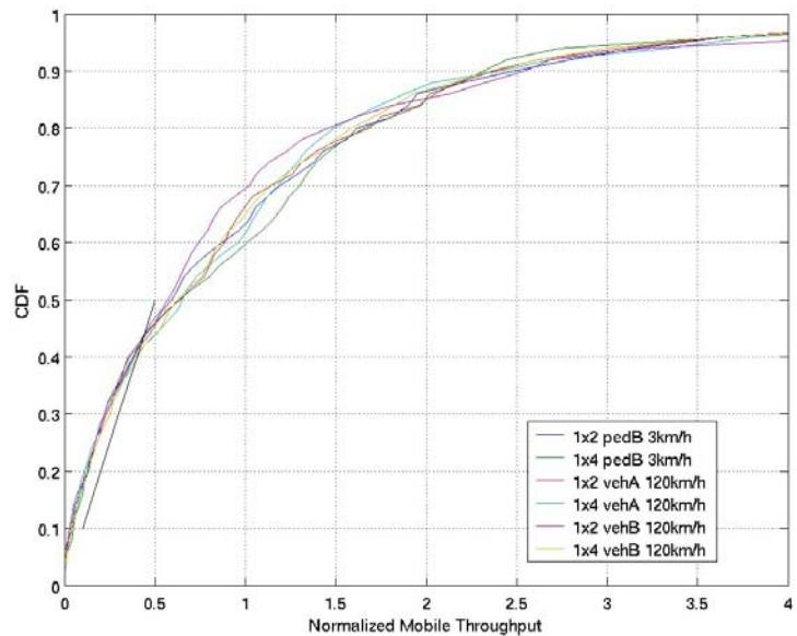
Figure6-4 フェアネス評価(UL, 2500m Site-to-Site Distance, 16 users per sector)
