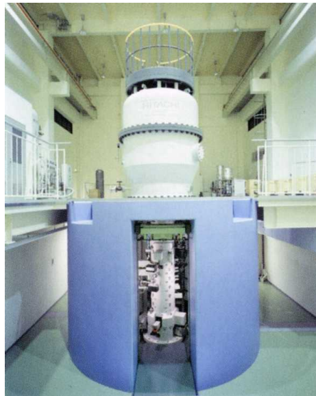
1MeV FE Electron Microscope developed by Dr. Tonomura's team at Hitachi ARL
