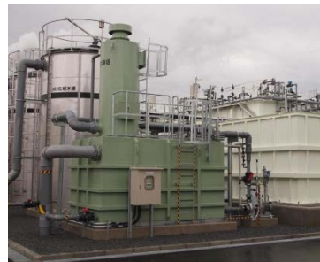
Sewage water membrane treatment system
