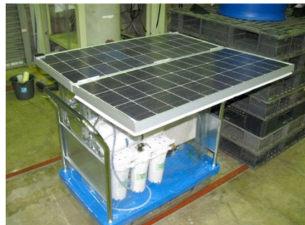
Installation of small solar-powered desalination machine (PVRO)
