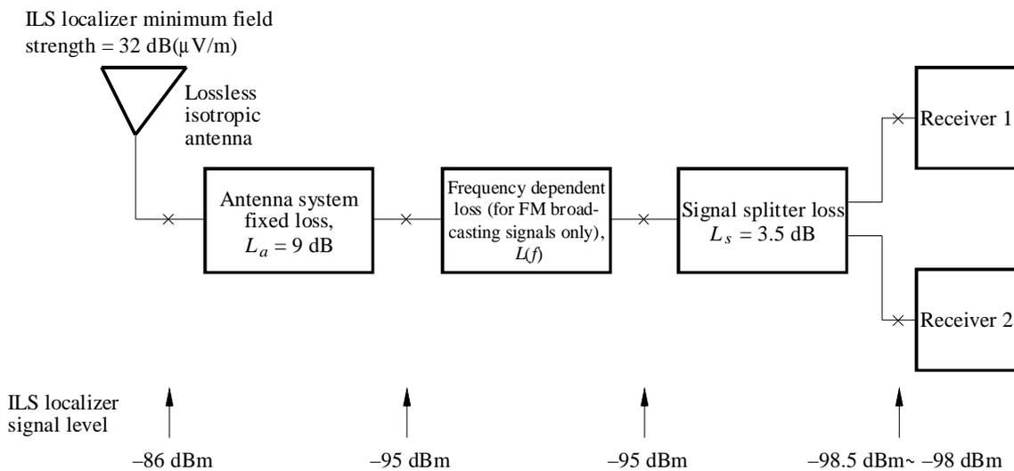
Note 1 – Typical aircraft installation includes a signal splitter to feed two aeronautical receivers.
