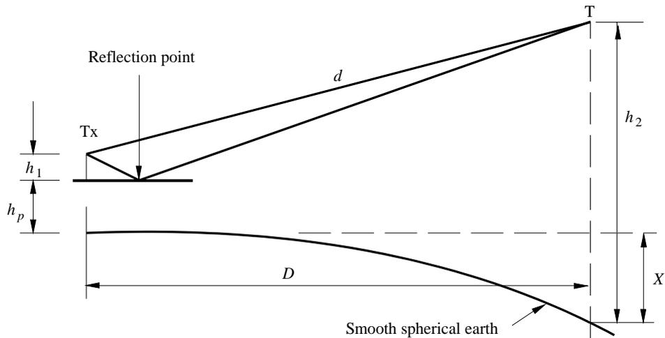
Note 1 – The effect of the Earth's curvature in the region between the transmitter site and the reflection point is neglected in this approximation.
