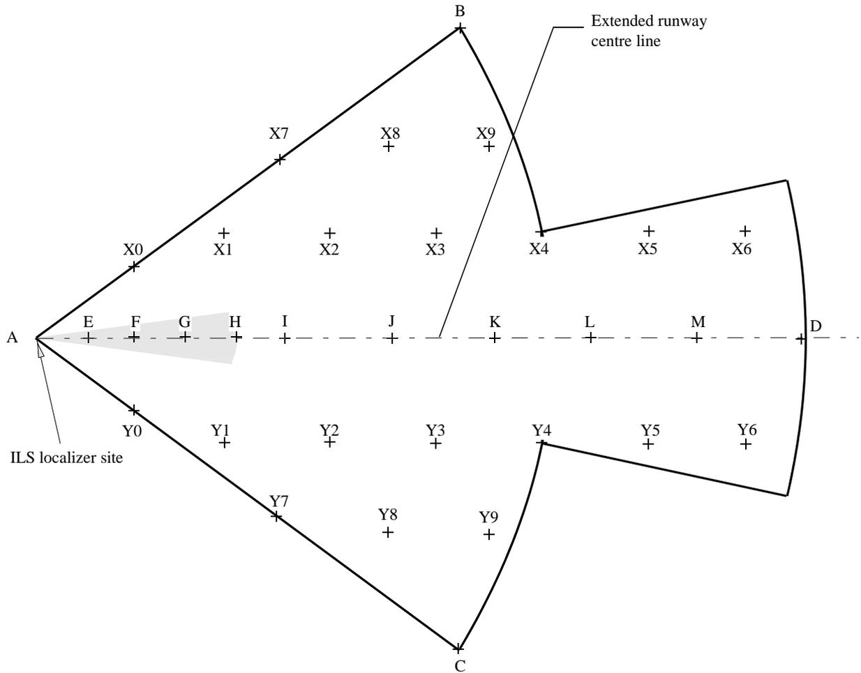
Note 1 – The shaded zone extends 12 km from the ILS localizer site and is within  $\pm 7.5^\circ$  of the extended runway centre line.
