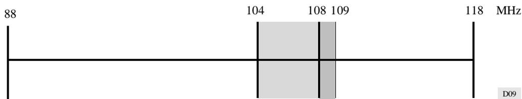
The frequency range within which the Montreal receiver may show more potential B1 interference than the GE84 receiver is shown shaded.
