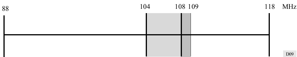
FIGURE 9 Spectrum chart for VHF/FM and ILS/VOR bands
