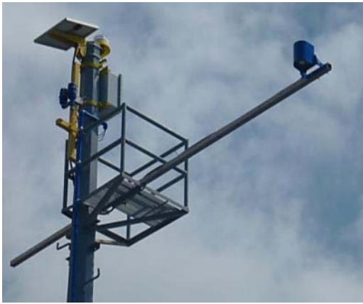
Mounted Ultrasonic Tide Sensor to continuously record the tide level
