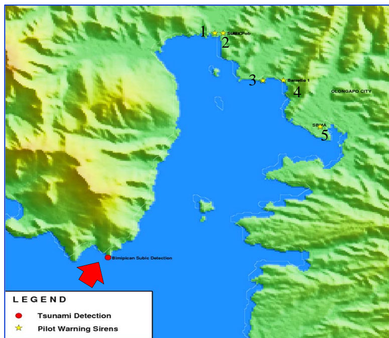
Ideally, Tsunami Detection Station is located far out the bay to provide more lead time to coastal communities like for Pilot Areas at Subic Bay: (1&2)Wawandue and Poblacion, Subic, Zambales, (3&4) Barretto, Olongapo City, and (5) SBMA.
