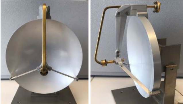
40dBi, 76,5GHz parabolic antenna 20cm diameter
