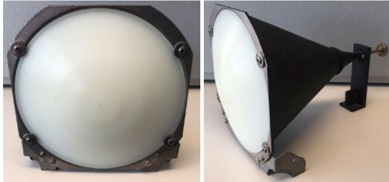
40dBi, 76,5GHz horn antenna 18cm diameter
