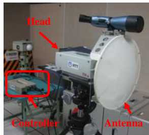
Figure 13 Composition of the 120-GHz-band radio equipment
