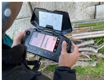
A machine to control drone (screen for checking the spots of inspection)
