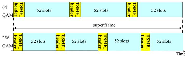
**[Figure C.4 Structure of super-frame for 64 QAM and 256 QAM.](#)**
