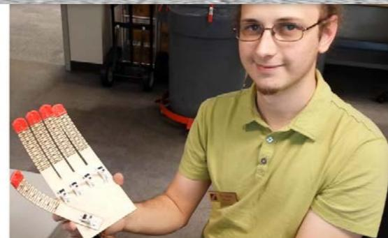
User controls robotic hand using custom flex sensors on glove
