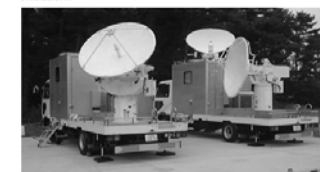
FIG 1. Photograph of developed multiparameter radar system. X-band (right) and Ka/W-band (left) radar subsystems are mounted on 4-ton truck. The antenna on the top of
