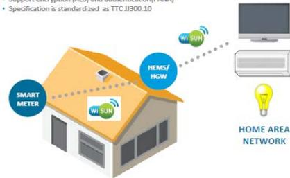
TEPCO B-ROUTE: Communication Between Smart Meters and HEMS      HAN: Communication between HEMS controller and HAN device
