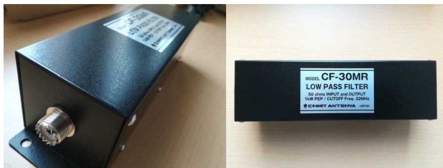
COMET社製 LPF CF-30MR Cut Off Freq = 32MHz
