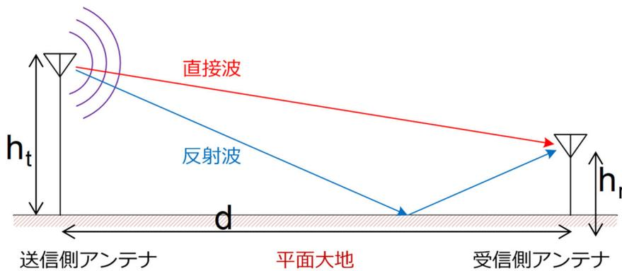
$$\begin{cases} L = \frac{1}{2} \left( \frac{\lambda}{2\pi d} \right)^2 & d < \frac{2\sqrt{2}\pi h_t h_r}{\lambda} \\ L = \frac{h_t^2 h_r^2}{d^4} & d \geq \frac{2\sqrt{2}\pi h_t h_r}{\lambda} \end{cases}$$
