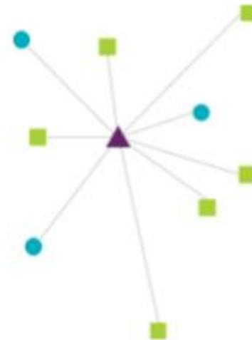
Licence authorises a base station at a given location (max EIRP 42 dBm) and any connected terminals.
