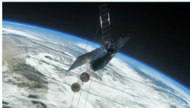
An Orbcomm satellite provides AIS communications to shipping (source: YouTube/Saab)
