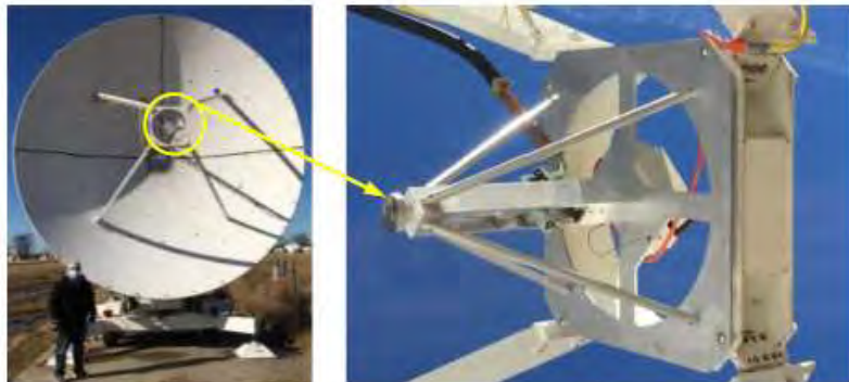
5.4m Parabolic Antenna with 10.5 GHz, 91.2kW Pulse Magnetron
