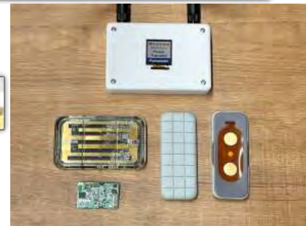
Receiver (Rectenna) < 1mW @ 10m
