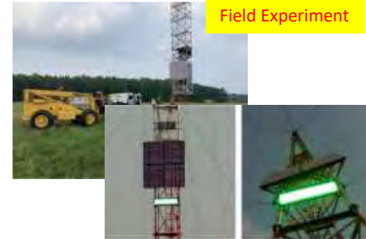
Field Experiment with 91.2kW-TxMW to 1.6kW-RxDC in > 1km in X-Band, by C. Rodenbeck, NRL, J. of Microwaves, 2022
