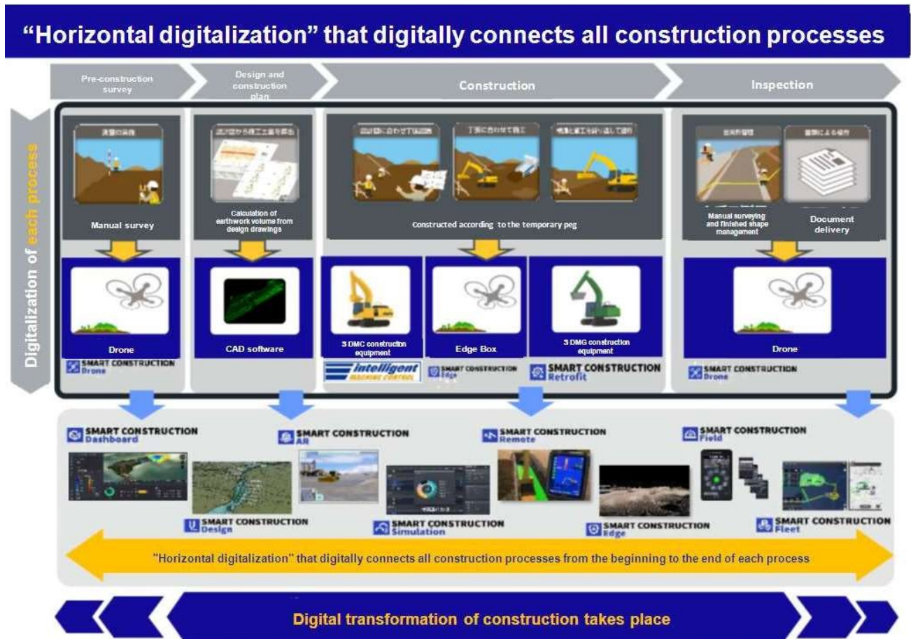
Figure 4-6 DX Smart Construction Concept
