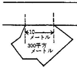
$$\begin{aligned} \text{奥行距離} &= \frac{300}{10} \\ &= 30(\text{メートル}) \end{aligned}$$
