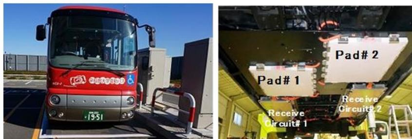
Figure 6. The Small Bus (WEB3 Advanced) and the Receive Equipment installed to the Bus.
