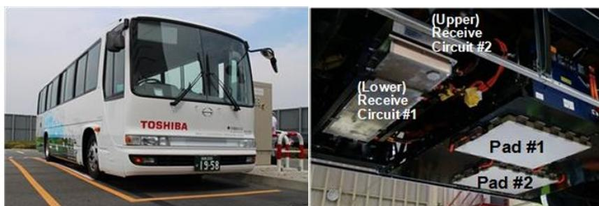
Figure 7. The medium-size bus and the receiving equipment installed on the bus.
