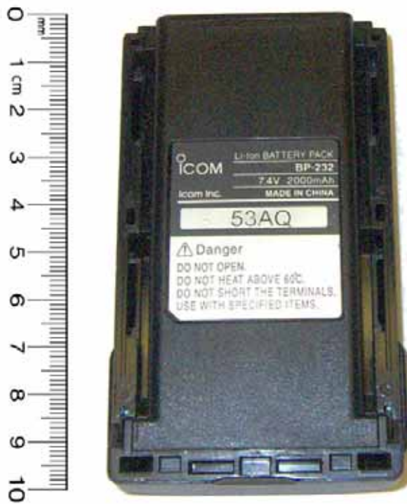
< Li-Ion battery pack (M/N: BP-232) >
