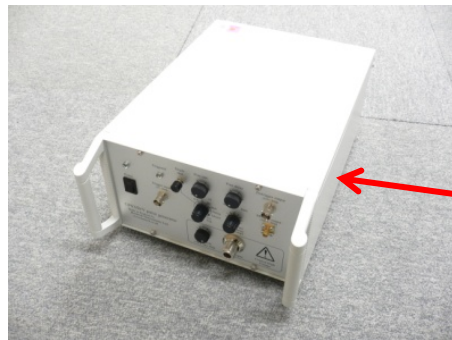
HIRA: Half reflector impulse radiating antenna
